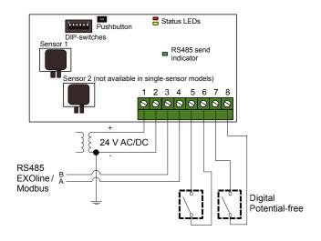
Fig. 3: Wiring with UIx as digital input
