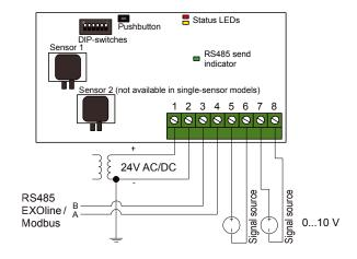
Fig. 2: Wiring with UIx as 0...10 V input
