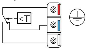
**Heating:** Connect to the red and blue terminal. The contact will open when the temperature rises..
