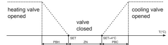
Inside the dead band (ZN) the regulator is in stand-by mode and the valves are closed, the fan is off. Outside the dead band, the regulation which is proportional is done on the heating valve if the temperature is lower than SET (setpoint) fixed with the knob, or on the cooling valve if the temperature is upper than SET+4°C.
