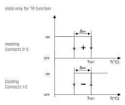
Ans: differential in the stage Tser: setting setpoint ON: closed contact OFF: open contact
