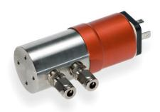
Transmitter for measuring differential pressure in liquids and gases. The method of measurement using a ceramic membrane gives a high level of accuracy and stability over a long period.
