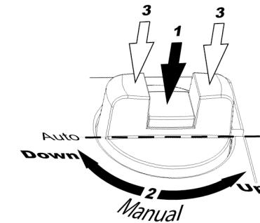
To manually set the valve position, first depress the central part of the button until it clicks and remains depressed (1 in the figure). This disengages the gears and also cuts the power to the motor. Then the valve position can be changed manually by turning the button (2 in the figure). Clockwise rotation will extend the drive rod and anti-clockwise will retract it.
