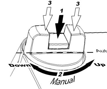
To manually set the valve position, first depress the central part of the knob until it clicks in place and remains depressed (1 in the figure). The valve position may then be changed manually by turning the knob (2 in the figure). Clockwise rotation will extend the drive rod and anti-clockwise rotation will retract it.
