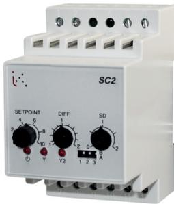
Suitable for heating/cooling or alarm applications. Convert a 0...10 Vdc input signal to a relay output. The controller are suitable for DIN-rail and have adjustable switching points. SC2 can be set to either binary or sequential control. Individually settable on/off levels.
