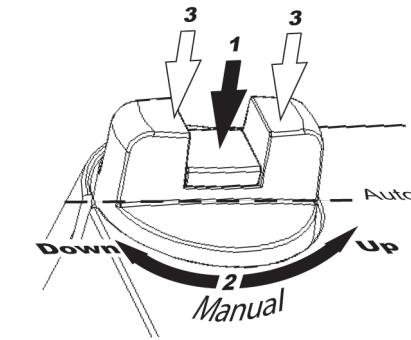
To manually set the valve position, first depress the central part of the button until it clicks and remains depressed (1 in the figure). This disengages the gears and also cuts the power to the motor. Then the valve position can be changed manually by turning the button (2 in the figure). Clockwise rotation will extend the drive rod and anti-clockwise will retract it.
