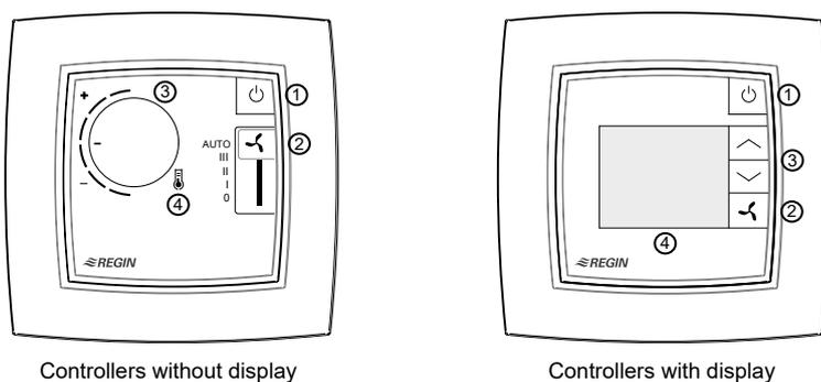
*Figure 4-1* Regio controller models without and with display
