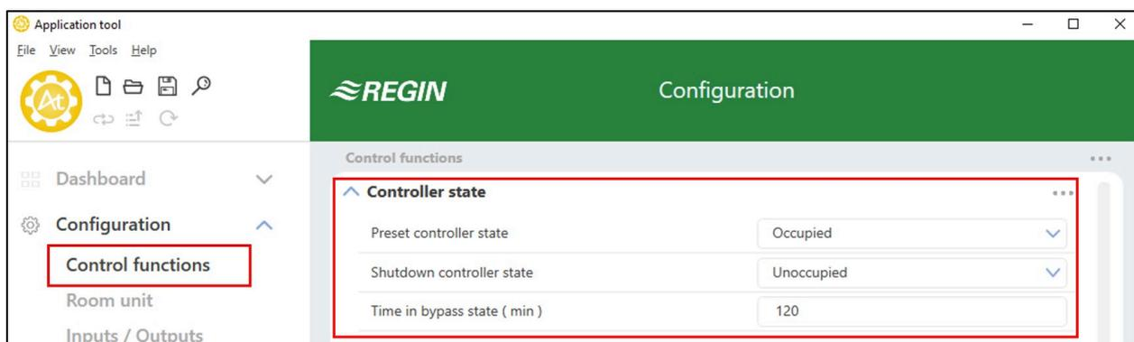
Figure 3-24 Controller state configuration settings in Application tool.
