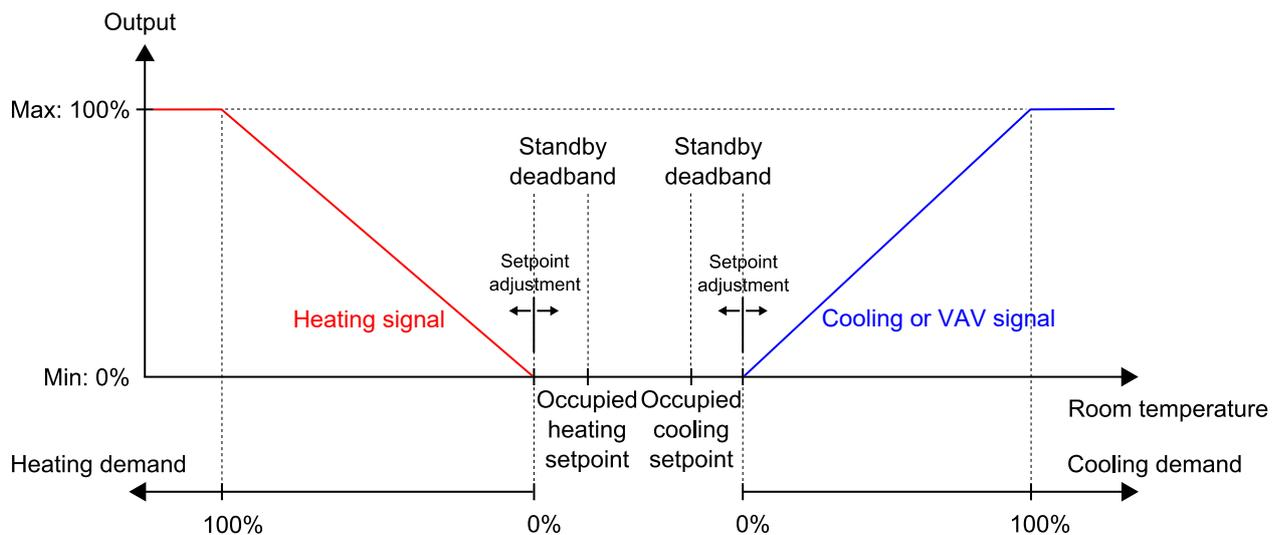
Figure 3-27 Control behaviour for the standby controller state.
