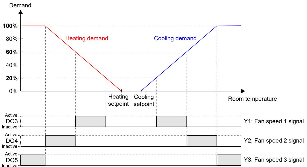
Figure 3-35 3-speed fan control behaviour in auto mode.
