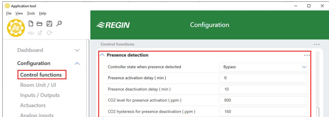
Figure 3-43 Presence detection configuration settings in Application tool.
