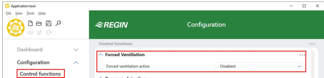
*Figure 3-41* Forced ventilation configuration settings in Application tool.
