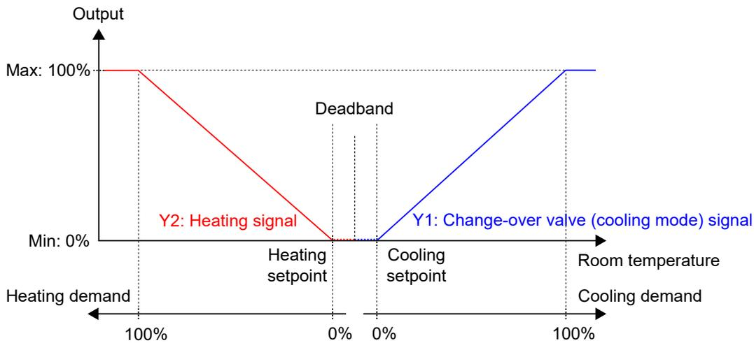
Figure 3-13 Control behaviour for the Heating + Heating/Cooling (change-over) controller mode when the controller is in Heating + Cooling mode.
