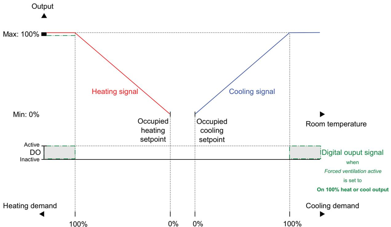
Figure 3-42 Example of forced ventilation control behaviour for the Heating + VAV controller mode when the controller is in bypass state.
