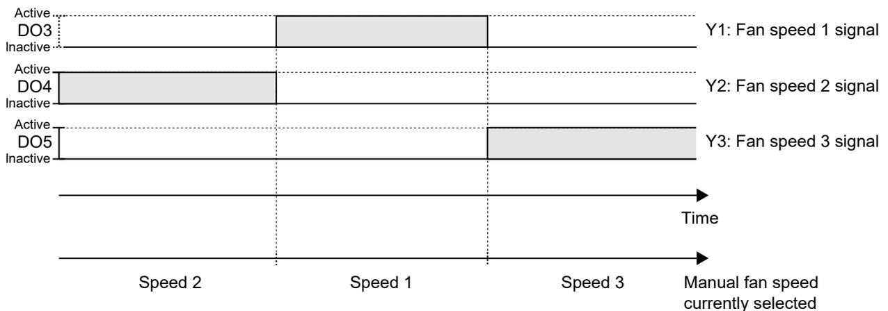
Figure 3-36 3-speed fan control behaviour in manual mode (fan speed 1, 2, or 3).
