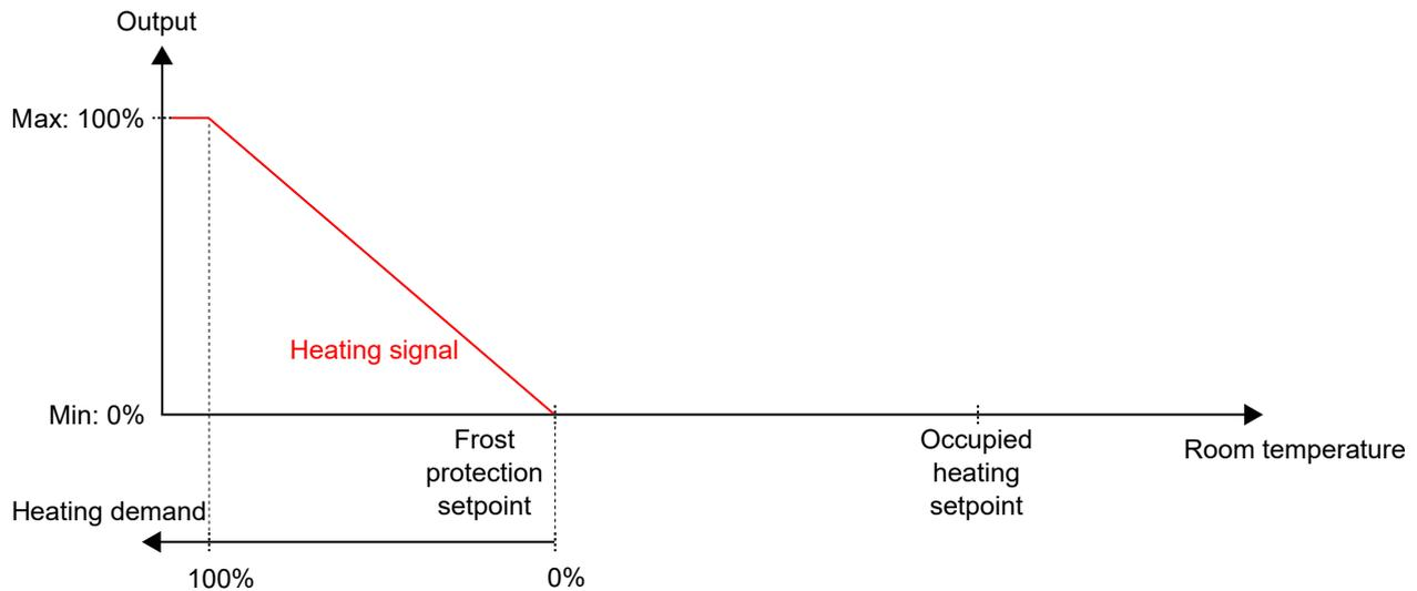
Figure 3-25 Control behaviour for the off controller state.
