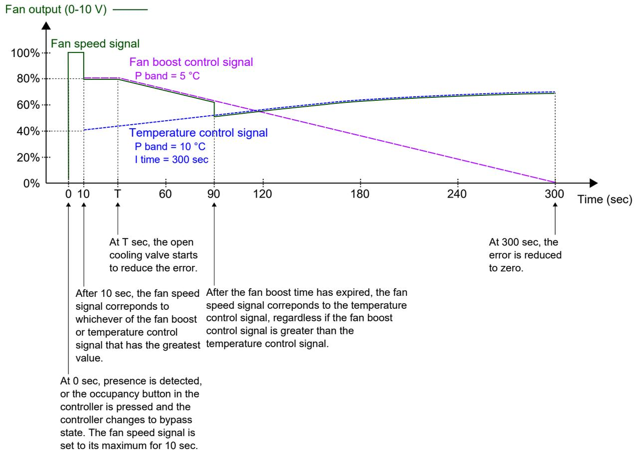
Figure 3-37 An example of fan boost control behaviour for an EC fan in auto mode, which provides a perceived cooling effect until the cooling distribution from the cooling valve establishes. The P-band for the fan boost controller has a lower value (higher gain) than the P-band for the temperature controller.
