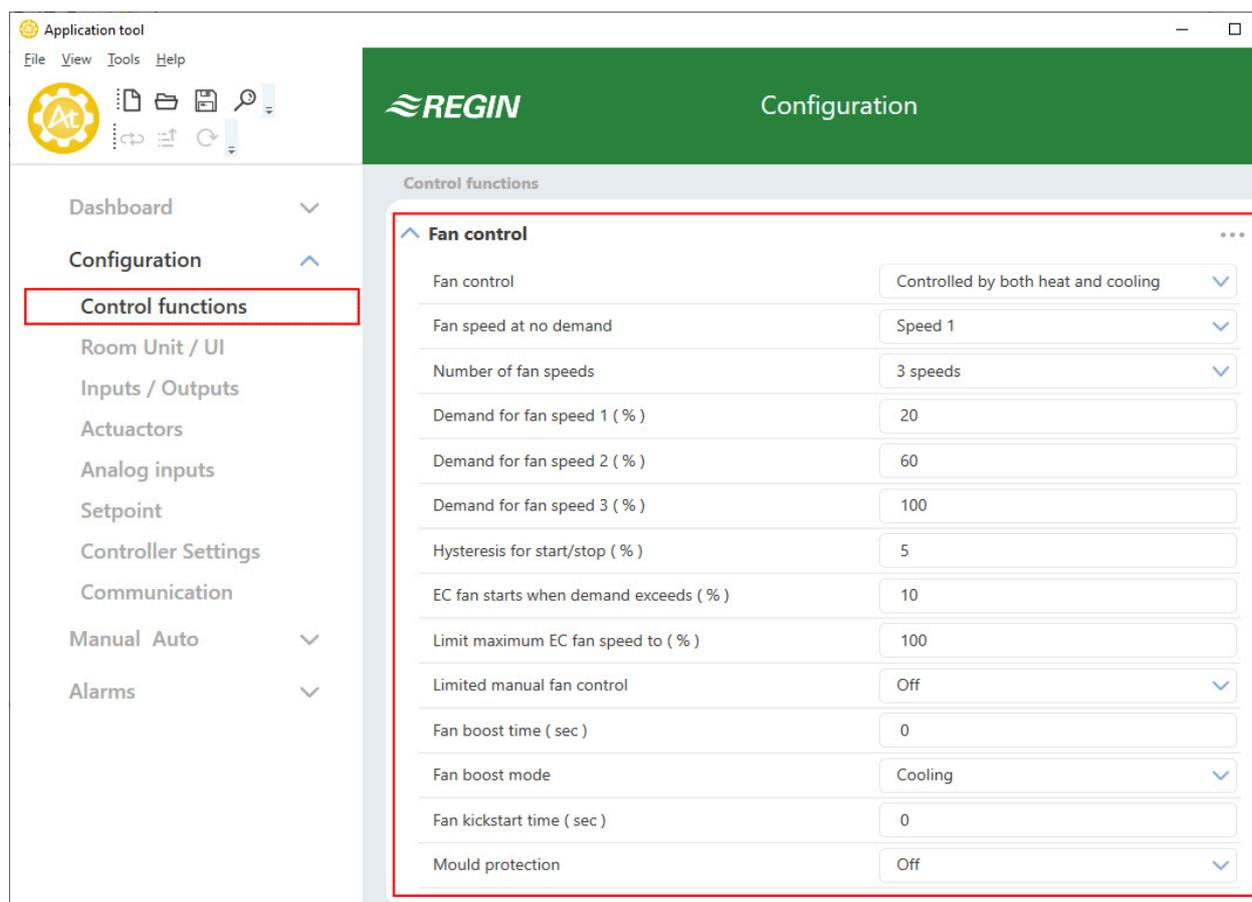
Figure 3-31 EC fan control configuration settings in Application tool.
