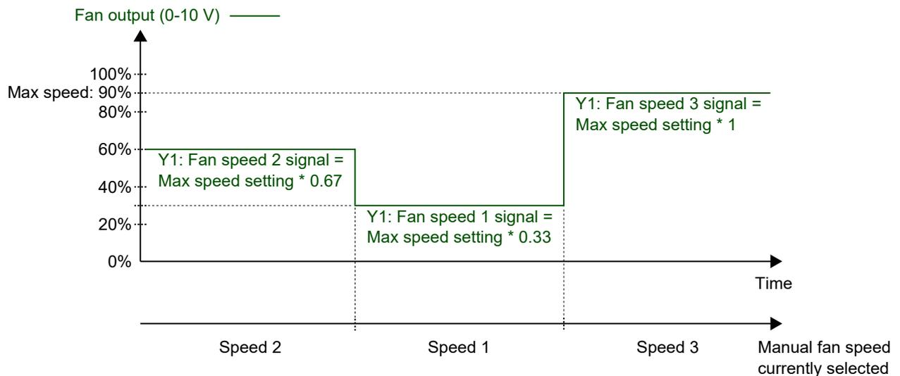
Figure 3-33 EC fan control behaviour in manual mode (fan speed 1, 2, or 3).
