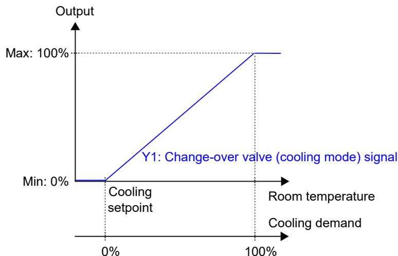
Figure 3-20 Control behaviour for the Heating/Cooling (change-over) controller mode when the controller is in cooling mode.
