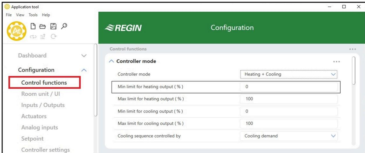
Figure 3-21 Configuration settings for minimum heating output limit in Application tool.
