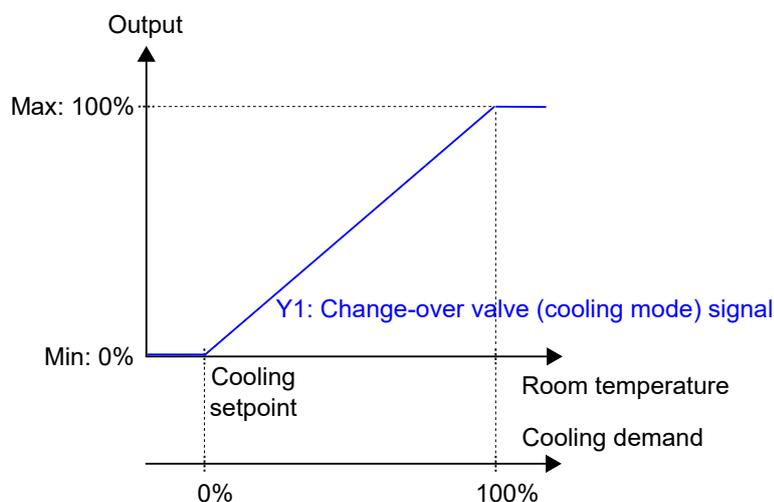
Figure 3-8 Control behaviour for the Heating/Cooling (change-over) controller mode when the controller is in cooling mode.
