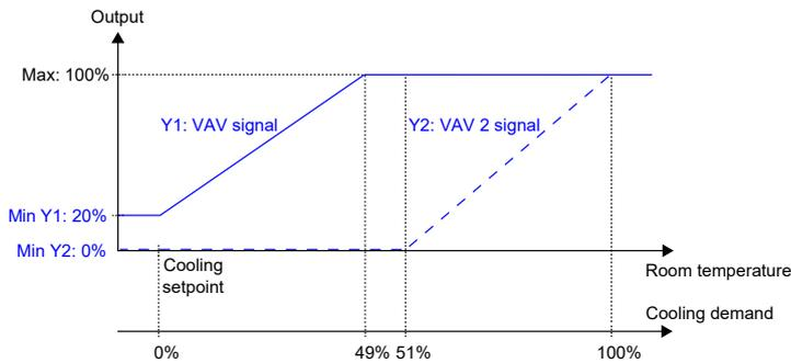
Figure 3-18 Control behaviour for the VAV + VAV controller mode when the controller regulates based on cooling demand.
