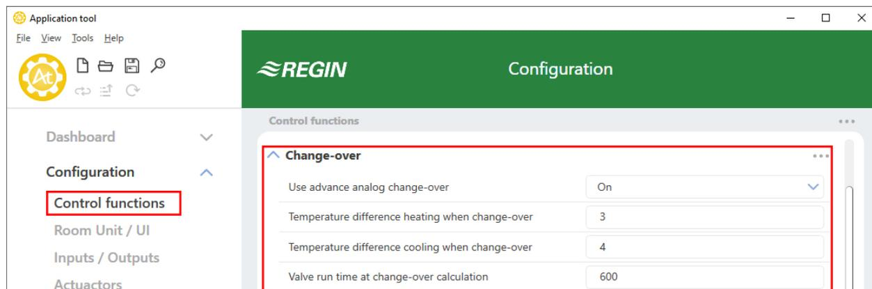
Figure 3-23 Change-over detection configuration settings in Application tool.
