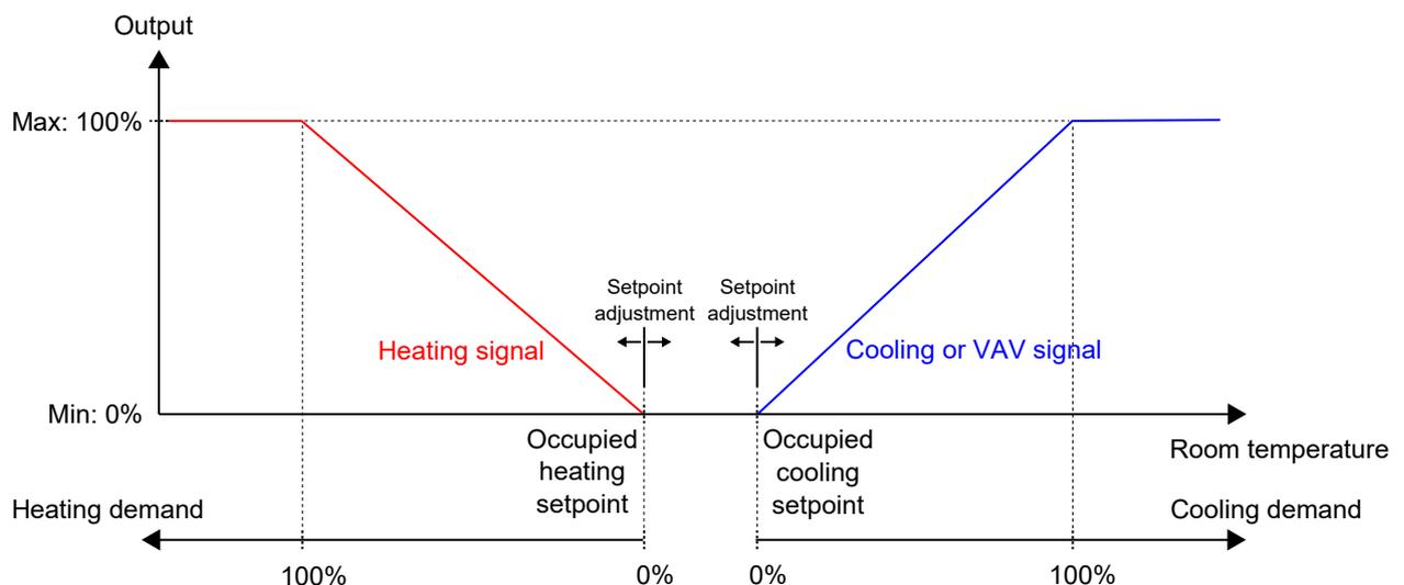
Figure 3-28 Control behaviour for the occupied and bypass controller state.
