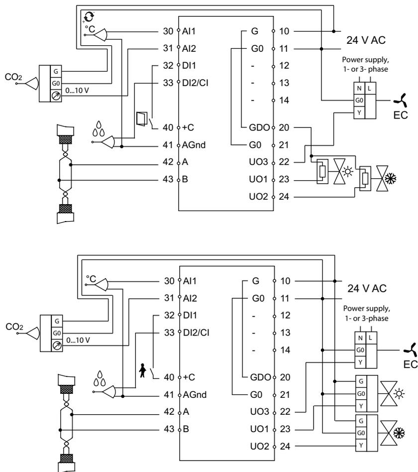
Figure 6-5 Connection diagrams for models for CO<sub>2</sub> control and fan control.
