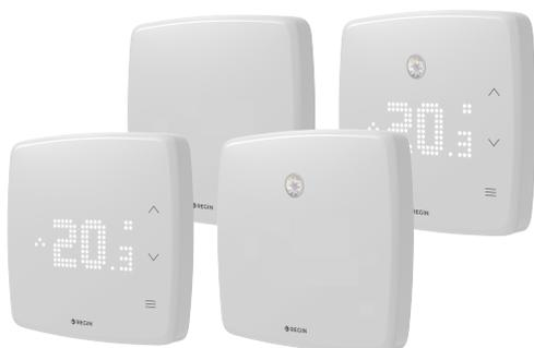
*Regio RCX series are controllers with built-in sensors and an RS485 communication port. Controllers in different rooms and zones can be connected to a field bus enabling communication with a central SCADA system, via RS485 (EXOline, BACnet, or Modbus). They can also be used as stand-alone controllers for control of heating and cooling in a single zone or room.*
