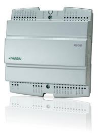
The RCP100... controllers are part of the Regio Maxi series. Since they have communication, they can be integrated into larger or centralized SCADA systems, e.g. EXOscada, if required. The controllers can be configured via the free software Regio tool<sup>®</sup> and freely programmed via EXOdesigner. They can be connected to Regio room units (RU-units) containing a built-in temperature sensor.
