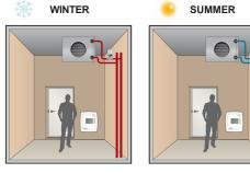
In 4-pipe installations, there are two separate water systems for heating and cooling with separate valves. The controller uses two outputs for control of heating and cooling in sequence.
