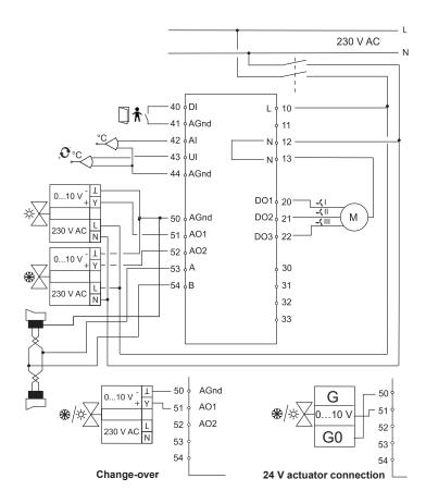
Automatic change-over between cooling/heating
