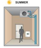
In 4-pipe installations, there are two separate water systems for heating and cooling with separate valves. The controller uses two outputs for control of heating and cooling in sequence.
