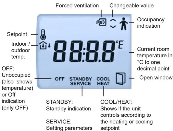
The buttons on the controller enables easy setting of parameter values using a parameter menu shown in the display. The parameter values are changed with the INCREASE and DECREASE buttons and changes confirmed with the occupancy button.
