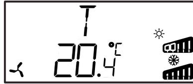
The upper row shows which control mode has been configured, in this case control mode 1, Temperature control, and the bottom row shows the actual value. The bar-graphs show the current output levels. In control mode 1, there are symbols showing how the outputs have been configured (Heating, Cooling, Damper or Change-over).
