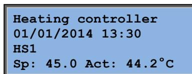
The display has 4 rows of 20 characters each. It has background illumination. The illumination is normally off, but is activated as soon as a button is pressed. The illumination will be turned off again after a period of inactivity.
